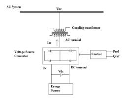
Fig 1: Functional block diagram of STATCOM
