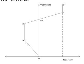
Fig 2: V-I Characteristics of STATCOM
