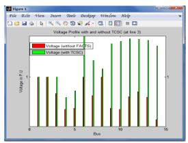
Fig 7: Voltage profile with and without TCSC (at weakest bus 3)
