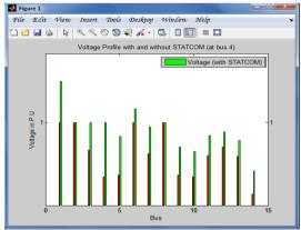
Fig 5: Voltage profile with and without STATCOM (in weakest bus 4)
