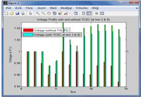
Fig 8: Voltage profile with and without TCSC at weakest bus 3 and weak bus 8
