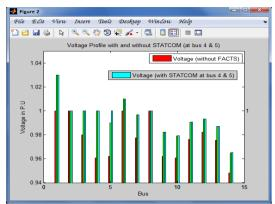
Fig 6: Voltage profile with and without STATCOM (at weakest bus 4 and weak bus 5)
